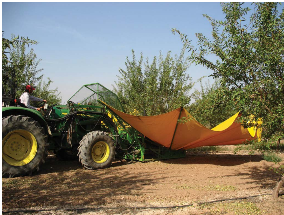
Fig. 17.13. A model M6 Almond shaker from Topavi (Autol, La Rioja, Spain) with an inverted umbrella for nut reception.
