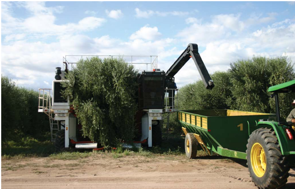
Fig. 17.12. A MaqTec Colossus® harvester from Maq Tec (Venado Tuerto, Sante Fe, Argentina) continuously harvesting 'Barnea' olives in Argentina. (Photo courtesy of L. Ferguson.)
