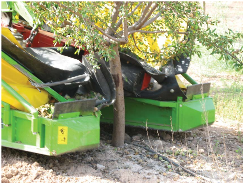
Fig. 17.3. Shaking head of a powerful multidirectional shaker.
