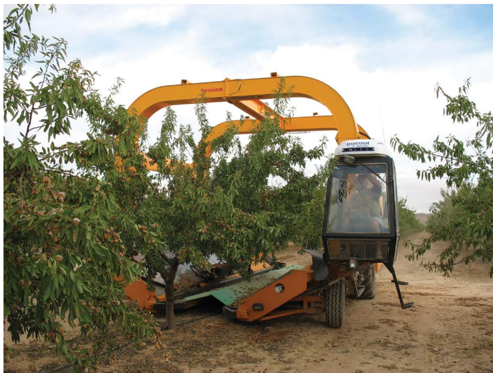
Fig. 17.11. Almond harvester under development by the manufacturer Tenías (Ejea de los Caballeros, Zaragoza, Spain).
