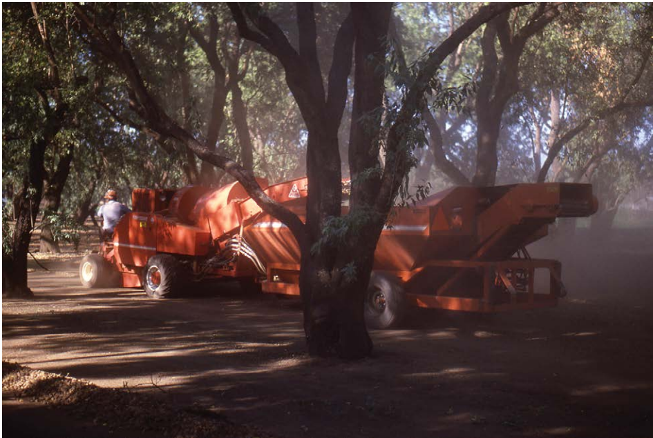
Fig. 17.6. A Flory model 6500 pickup machine (Flory Industries, Salida, CA, USA), towing a conveyor cart from Thomas Manufacturing Co. (Chico, CA, USA), picks up a row of nuts, separates leaves, twigs and soil and leaves debris behind in the field while loading the conveyor cart.
