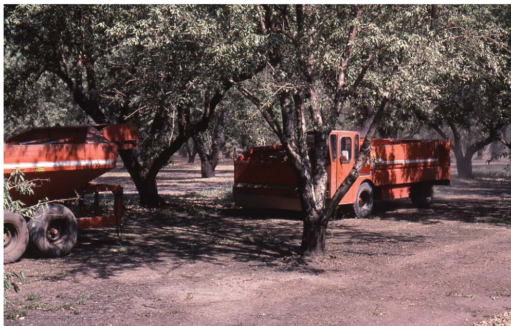
Fig. 17.7. A nut Bankout shuttle wagon from Thomas Manufacturing Co. (Chico, CA, USA) approaches a conveyor cart to offload accumulated nuts for transport from the orchard for hulling.
