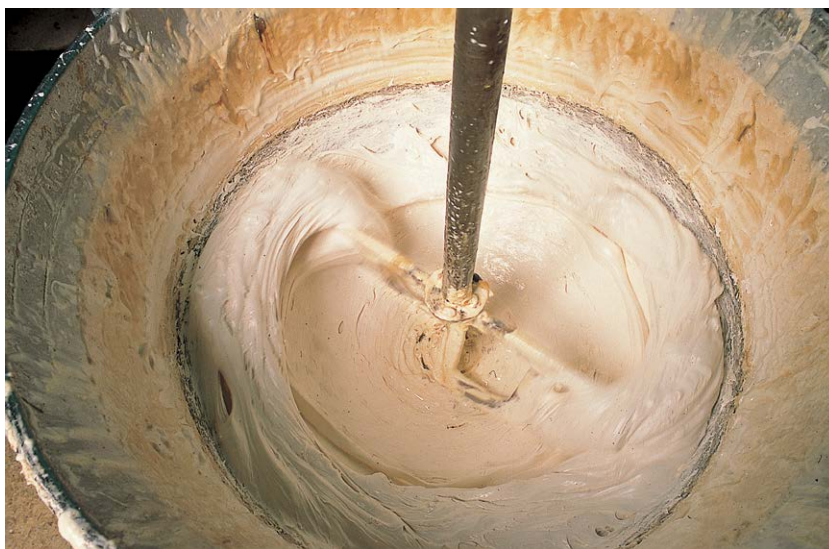
Fig. 20.10. Mechanical cooking of sugar, honey and egg white. (With kind permission from RCPGIJA, http://www.jijona.com .)
