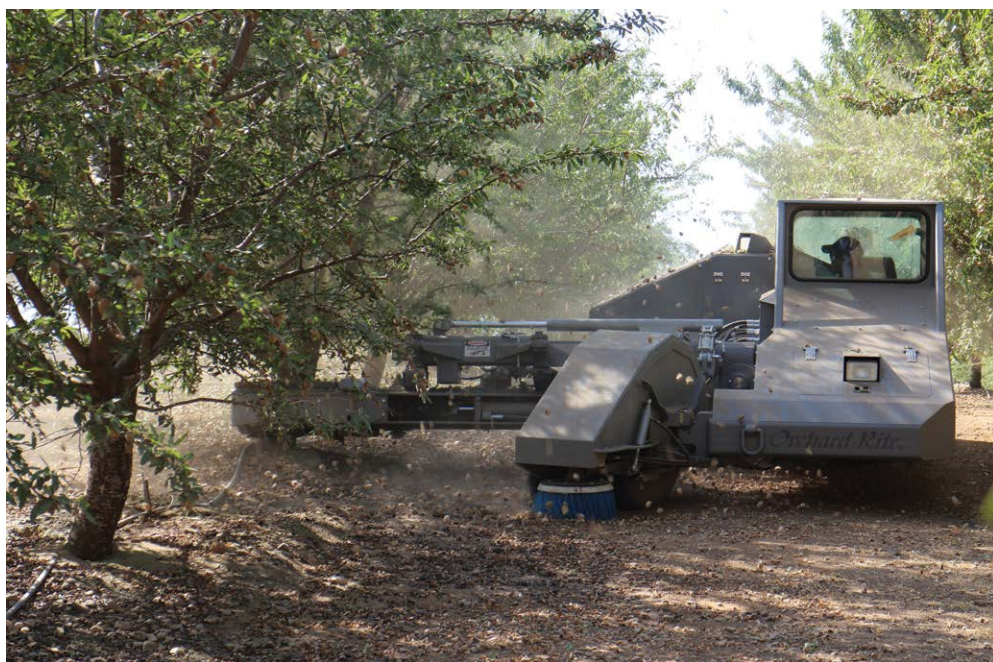
Fig. 179. The Orchard-Rite® Bullet®, a self-propelled side-mounted tree shaker can move rapidly down the tree row working quickly and effectively on trees that can be trunk shaken. (Photo courtesy of Orchard-Rite®.)
