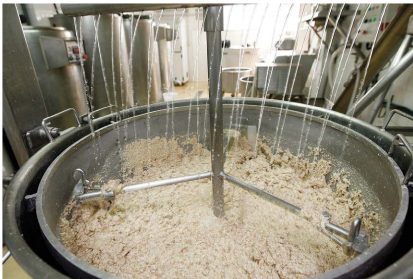
Fig. 20.17. Sieve press for 'horchata' preparation. (With kind permission from TDC Association, http://www.tdc.es .)
