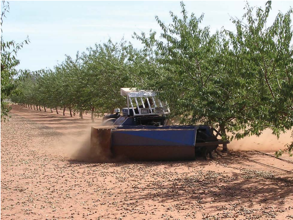
Fig. 17.5. A Weiss McNair (model JD-80) mechanical sweeper blows nuts from the tree row and sweeps nuts into a row in the orchard middle. (Photo courtesy of Weiss McNair, Chico, CA, USA.)
