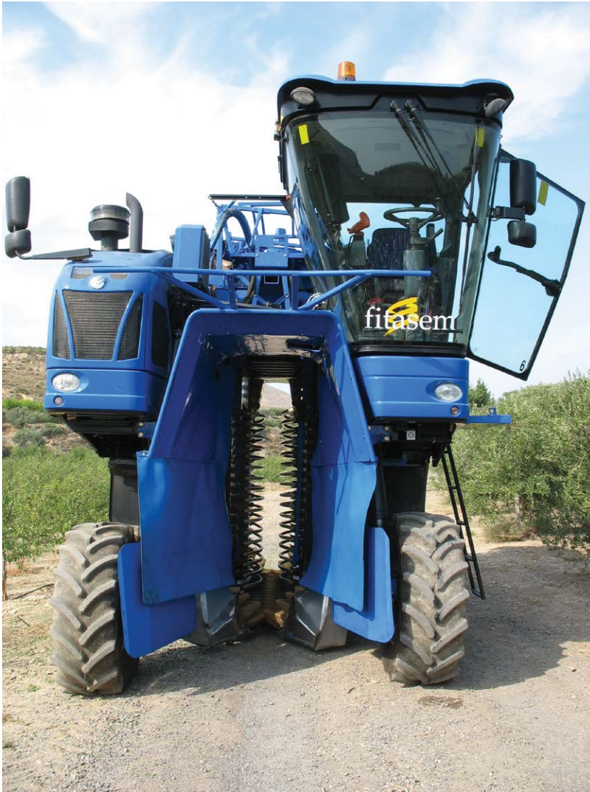
Fig. 17.10. Almond harvester adapted from grape harvesters, under development by the manufacturer Fitasem (Barbastro, Huesca, Spain).
