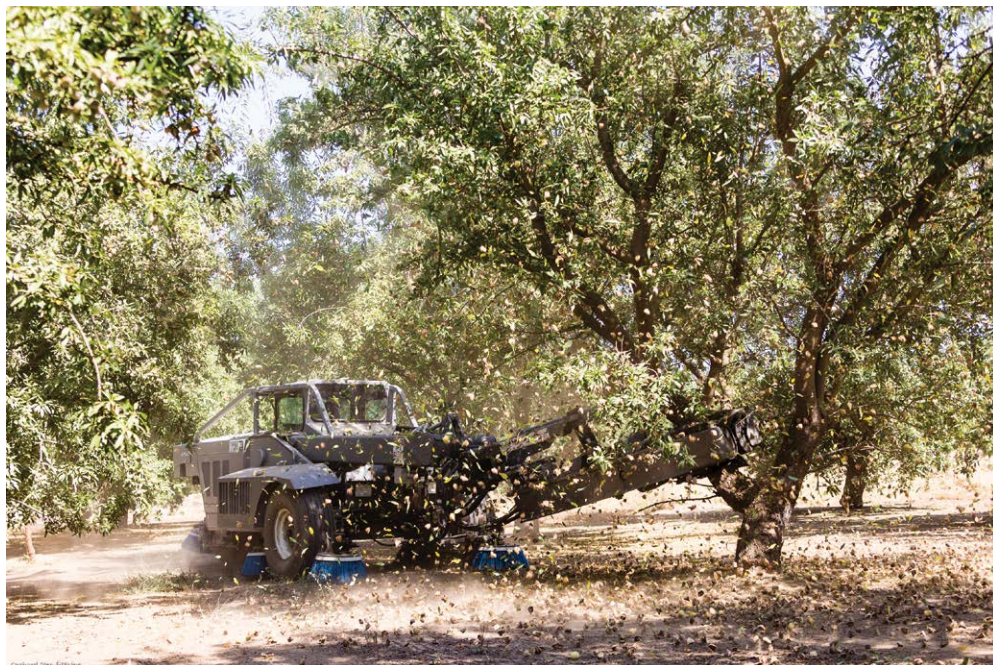
Fig. 178. This self-propelled Monoboom® shaker from Orchard-Rite® (Yakima, Washington, USA) will effectively handle either trunk or limb shaking as needed. (Photo courtesy of Orchard-Rite®.)
