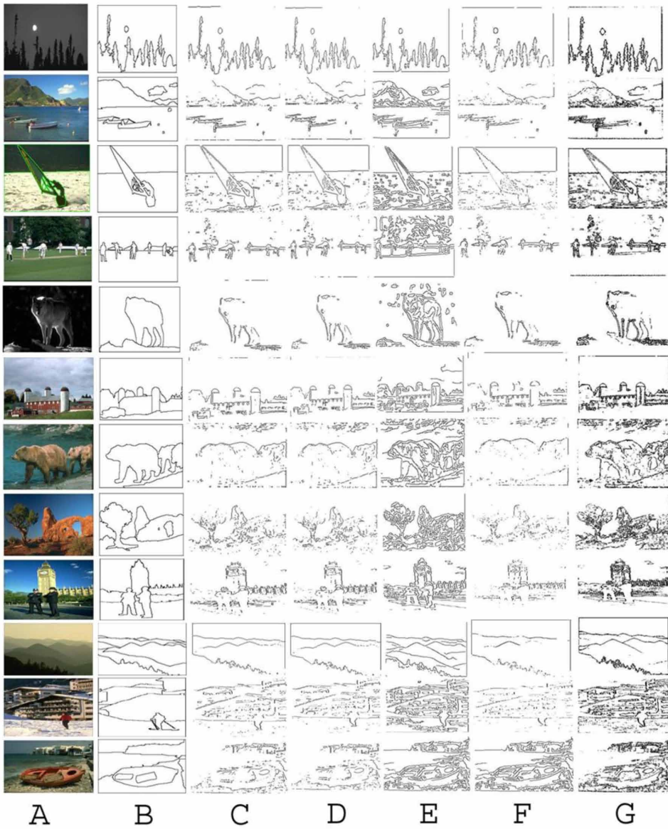
Figure 18. (A) Original Image (B) Human Segmented (C) Sobel (D) Prewitt (E) Canny (F) Roberts (G) Proposed
