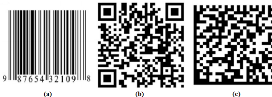
Figure 2. Three popular barcode patterns: (a) Universal Product Code (UPC), (b) quick Response code (QR code), (c) data matrix. (Reproduced from Chen et al.[61] with the kind permission of the Publishers).
