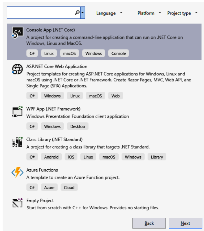
Figure 1.7 – Select the Console App (.NET Core) template when creating a new project in Visual Studio
