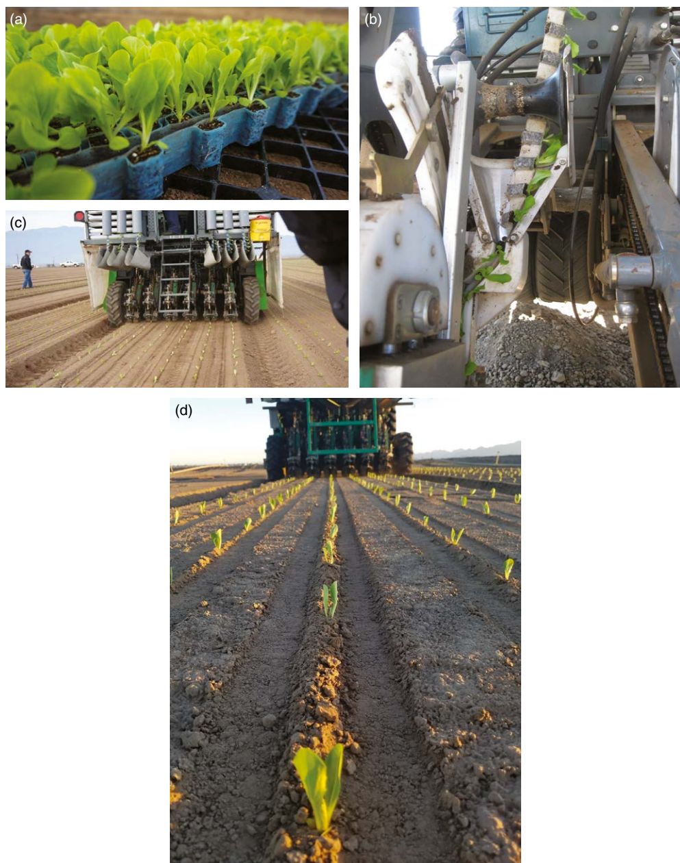
Fig. 2.9. Integrated PlantTape® System: (a) lettuce transplants growing in a tape; (b) automatic discharge; (c) transplanting with multi-row capacity; and (d) field establishment.
