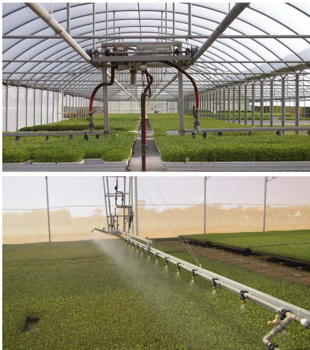
Fig. 2.3. Overhead irrigation system for greenhouse vegetable transplant production. Watering nozzle arms attached to a semi-automatic assembly are suspended on trellis in the center of the greenhouse. Production system with a T-rail benches (top) and wire railings (bottom) for tomato transplants.
