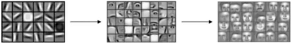
Figure 2.14: An illustration showing that deep layers learn high-level features and shallow layers learn low-level features.
