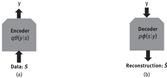
Figure 5.2: (a) The encoder is used to compress data into latent space ( y ). (b) The decoder is used for reconstruction of given data which is a hidden representation.
