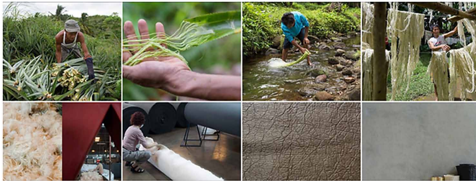
Figure 14. Pinātex manufacturing process: harvesting, dismantling, drying, washing, degreasing, fabric formation, finishing, final fabric
