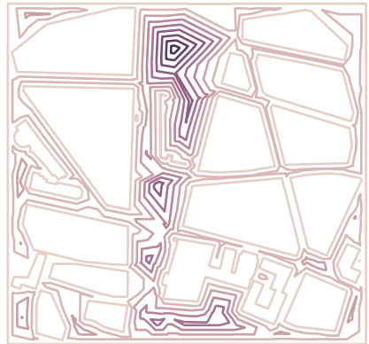
b) Distance function \hat{d}_\Omega which gives the minimal distance to the nearest obstacle.
