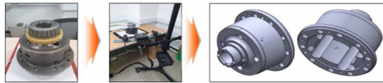
Figure 2. Automobile differential gear case reverse engineering process (Source: Metal3D)
