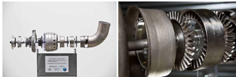
Figure 1. The world's first 3D printed prototype of jet engine that was on display at Paris Airshow-2015 (Adapted from https://www.monash.edu/mcam/news/articles/paris-le-bourget-airshow (Wu, 2015); Used with permission from MCAM, Monash University, Australia).
