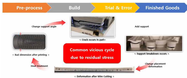
Figure 13. Problems of metal AM part manufacturing, all images courtesy of ANSYS (Source: ANSYS)
