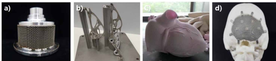
Figure 3. Definition of DfAM: a) Light weight b) Part unification c) Multi-property material d) Specialized part (Medical)
