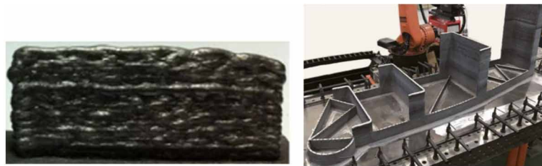
Figure 5. (a) Simple and (b) complex metallic parts produced via GMAW based AM process (Accessed under open access from Klobčar et al., 2018; Ma, Zhao, Li, Yang, & Xiao, 2019).
