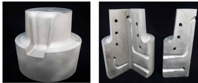
Figure 6. Mold printed with a 3D printer (Source: Metal 3D)
