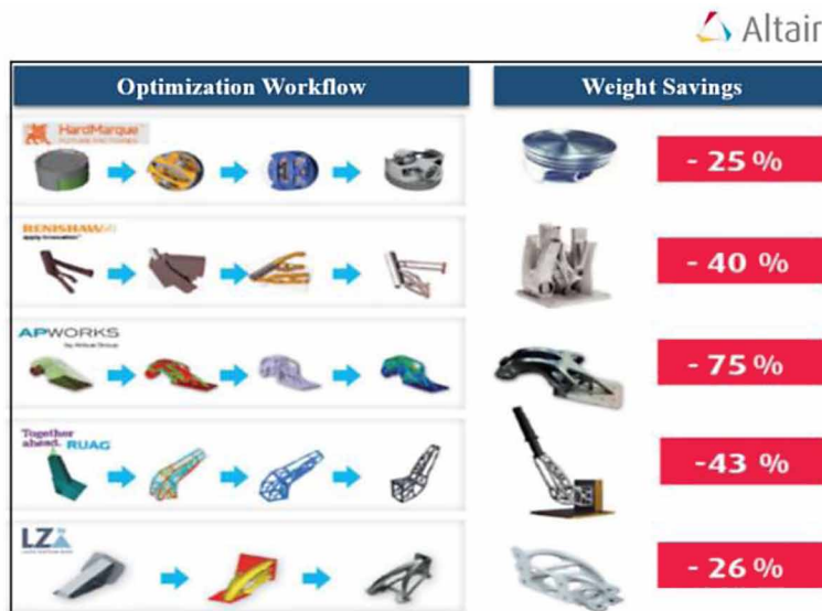
Figure 10. Example of implementation of topology optimization and lightweight by using INSPIRE, all images courtesy of Altair (Source: Altair)
