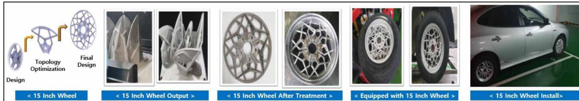
Figure 4. Car wheel applied with DfAM Design Technology (Source: KAMUG & Metal3D)
