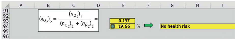
Figure 2.5: Calculation of the oxygen concentration and application of the Excel SI function.
