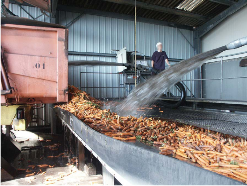
Fig. 15.3. Carrots being washed before entering the packing station. (Photo by E. Geoffriau.)
