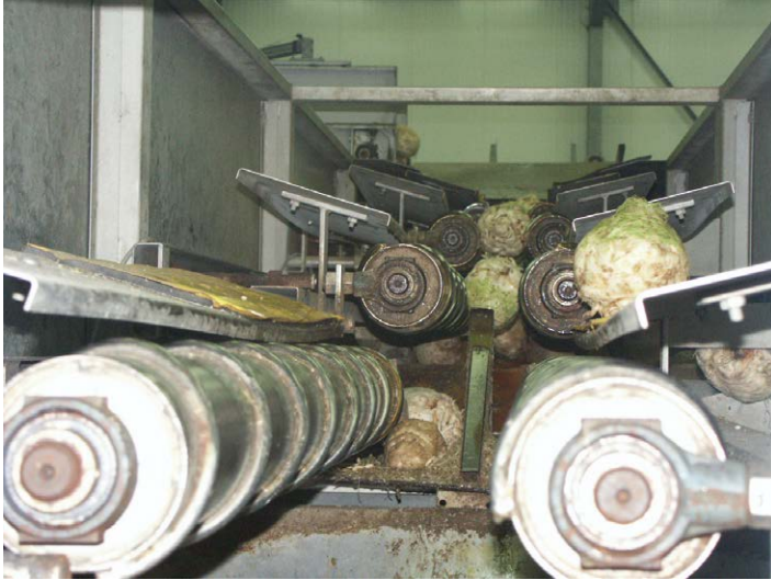
Fig. 22.5. Mechanical celeriac trimming. (Photo by E. Geoffriau.)
