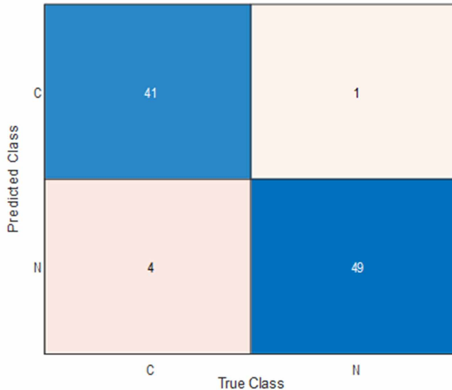
Figure 2. The confusion matrix that was obtained for ResNet50 and linear SVM classifier
