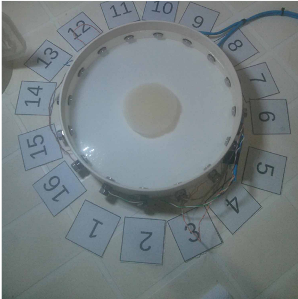
Figure 4. phantom environment with the 16 electrodes Source: The authors
