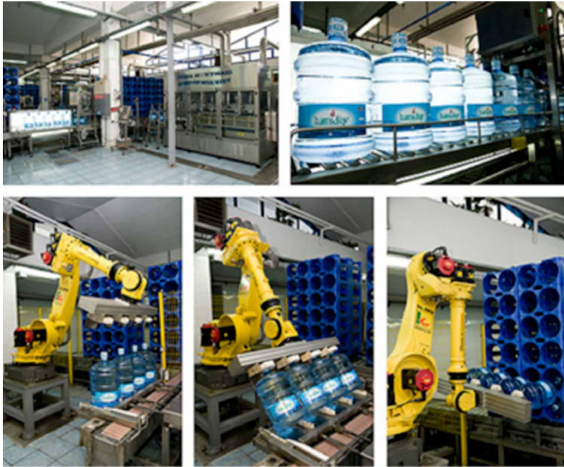
Figure 3. 19 liters HOD-demijohn water production line of the company
