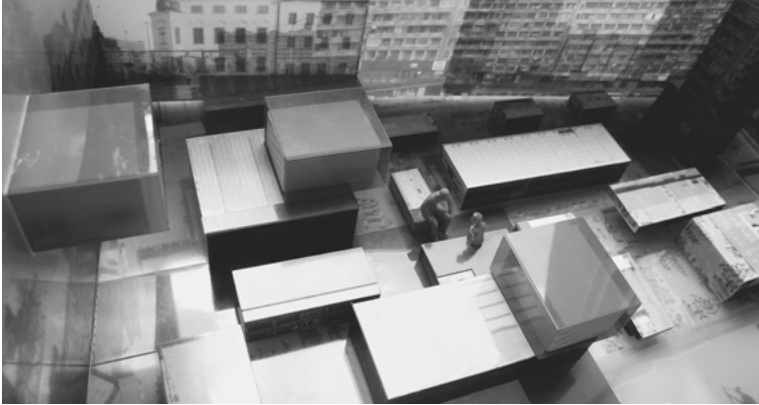
Fig. 48: Spatial presentation using projections of structural images onto the model to check and assess the spatial intervention.
