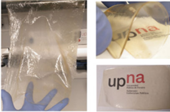
Figure 4.1: Transparent films prepared from wool keratin using sunflower oil (left) as plasticizer compared to glycerol (right) (Fernández-d’Arlas, 2019). Reproduced with permission through Open Access publication.
