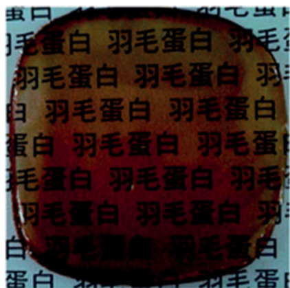
Figure 4.4: Transparent films were obtained by combing feathers with dialdehyde starch (Dou, 2015). Reproduced with permission from Royal Society of Chemistry.
