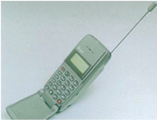
Figure 10.2: Core wire of NiTi alloy for cellular phone's antenna [20].
