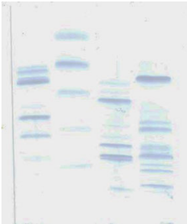
Figure 2.16-12: Semidry blotting of proteins in a TRIS-formate-taurinate buffer system after SDS disc-electrophoresis in a 713-SDS net gel. The blotting was carried out at constant electric current of 1 mA/cm 2 for 30 min. Amido black staining.
