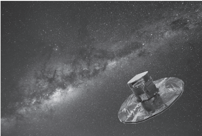
Figure 15-4. The spaceborne observatory Gaia, tasked with measuring the position, brightness, colours, spectra and velocities of a billion stars. Credit: ESA/ATG Medialab; background image: ESO/Brunier.
