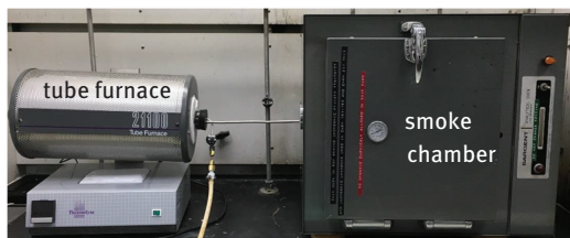
Figure 8.2: Smoke chamber setup. The outflow of the tube furnace (where the biomass is combusted) is directed into the smoke chamber (where residential materials are exposed).
