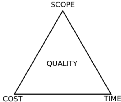
Figure 1.3 – The famous Iron Triangle of Project Management (also known as the Triple Constraint)
