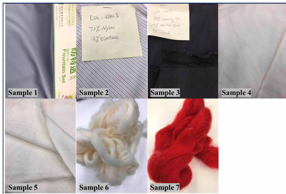
Figure 12. Using NIR to identify different textile material
