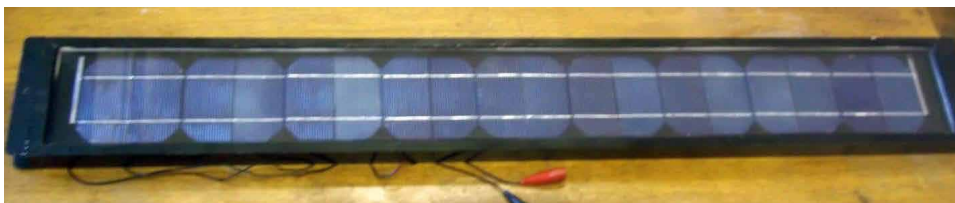
Figure 2. Produced thermal photovoltaic receiver concentrator solar installation
