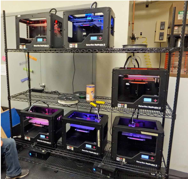
Figure 1. Example of a university build farm featuring FFF machines managed by a central system
