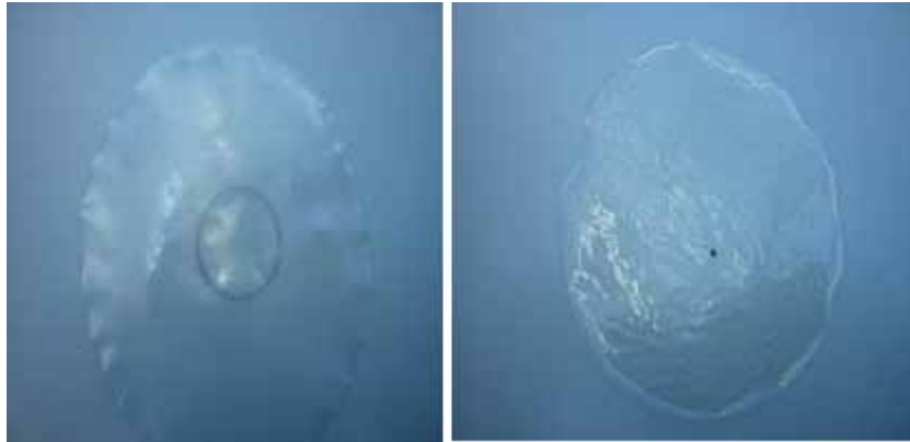
Figure 4. Photo for lab-tested samples under DC electric field breakdown for nanocomposite of Polyvinyl Chloride PVC with 10% Fumed Silica
