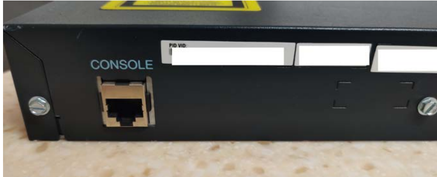
Figure 2.30 – Console port on the back of a Cisco IOS router
