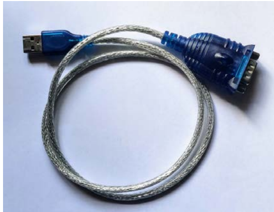
Figure 2.29 – USB to RS-232 converter cable
