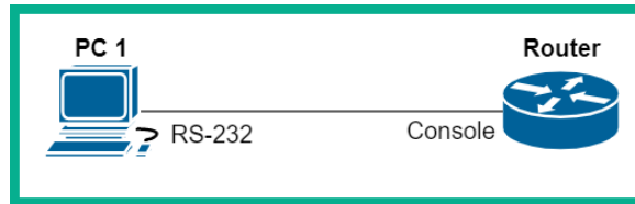
Figure 12.1 – Console lab topology
