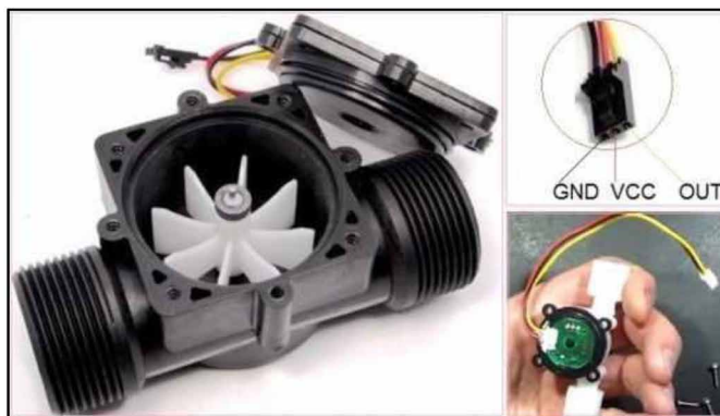
Figure 7. YF-S201 Hall-Effect Water Flow Sensor
