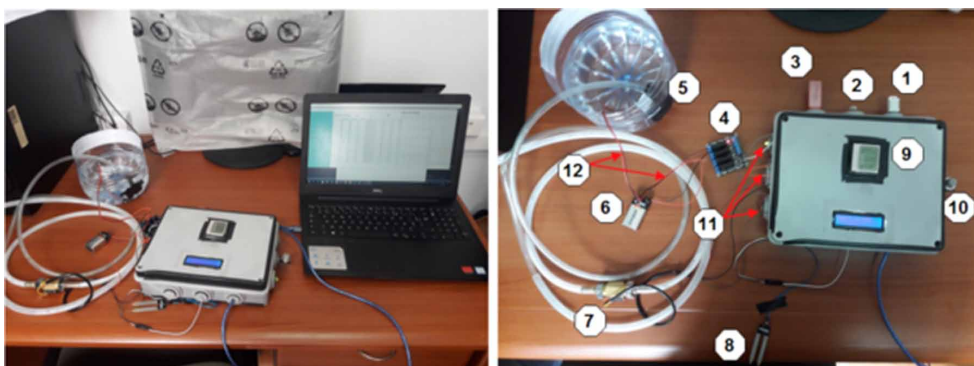
Figure 5. Field data collection device. [Legends 1: DHT22 Sensor, 2: LDR Sensor, 3: Water level Sensor, 4: Relay Switch, 5: Water pump, 6: Power supply 9 V, 7: Water flow sensor, 8: Soil moisture sensor, 9: LCD display, 10: MQ2 sensor, 11: LEDs, 12: Jumpers]. The mega Arduino card and NRF module are in the Box
