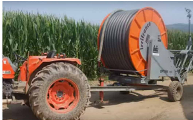
Figure 27. Gun sprinkler system (mounted on tractor)
