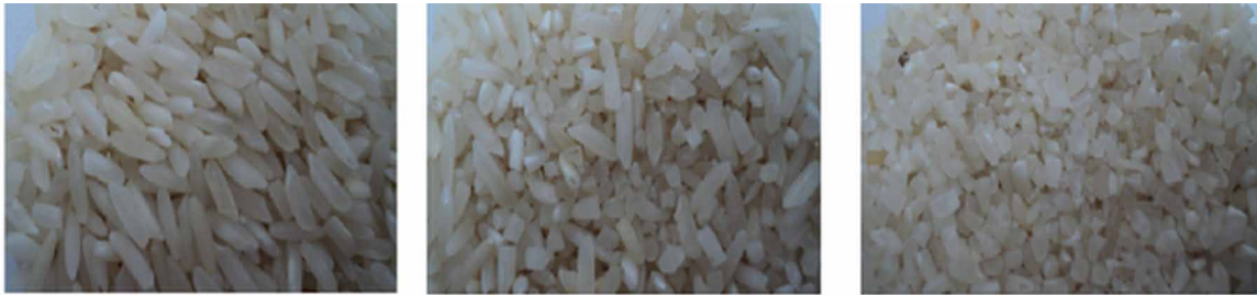
Figure 43. The rice grain with (a) 0%, (b) 50% and (c) 100% broken rate
