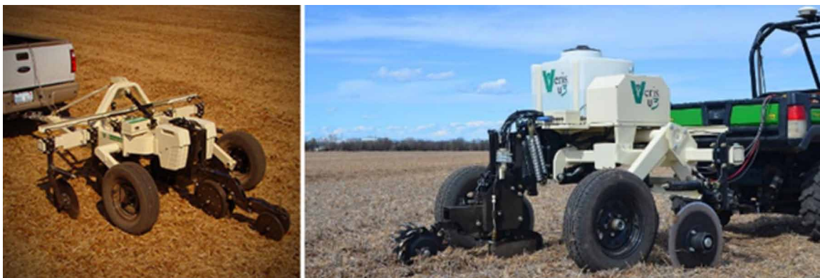
Figure 9. Examples of On-the-go sensors (Veris, 2014)
