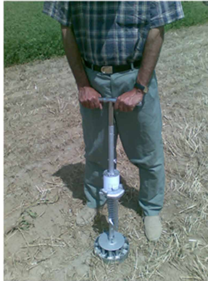
Figure 2. Picture of the shear ring apparatus in the field, (a) and illustration of device parts (b)
