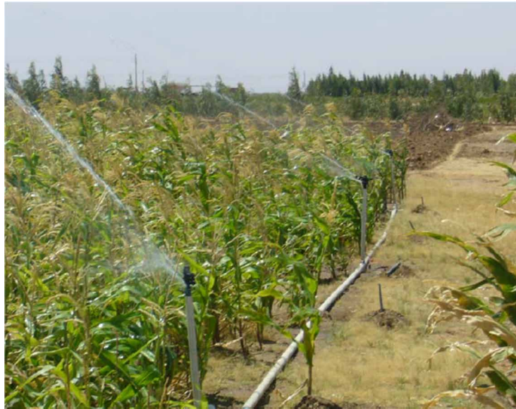
Figure 22. Semi-portable sprinkler irrigation systems
