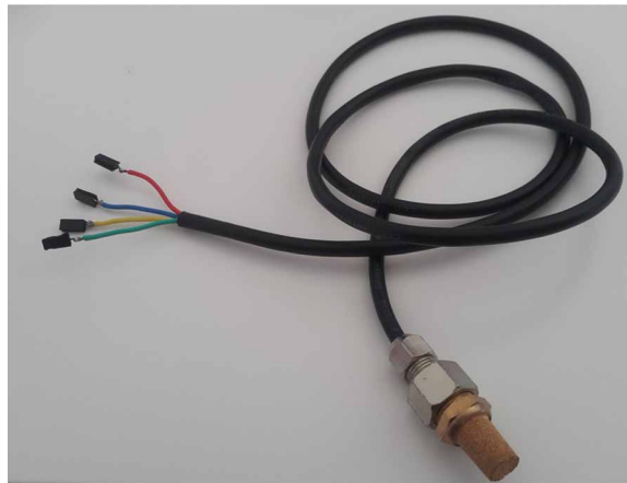
Figure 4. SHT-10 temperature and moisture sensor
