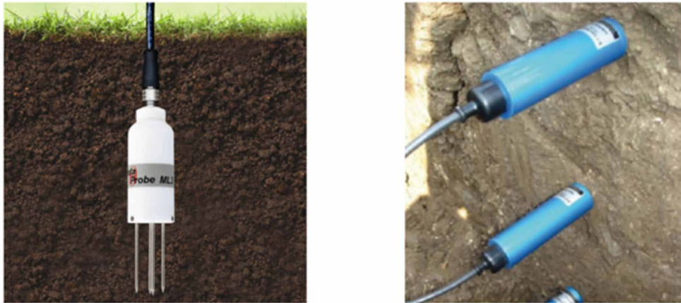
Figure 11. Delta-T ML3 probes for soil water content monitoring (Delta-T Devices Ltd, 2017)
