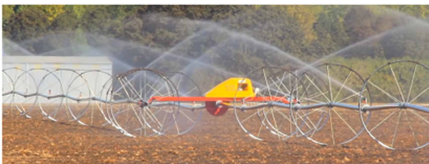
Figure 24. Side wheel roll sprinkler irrigation systems
