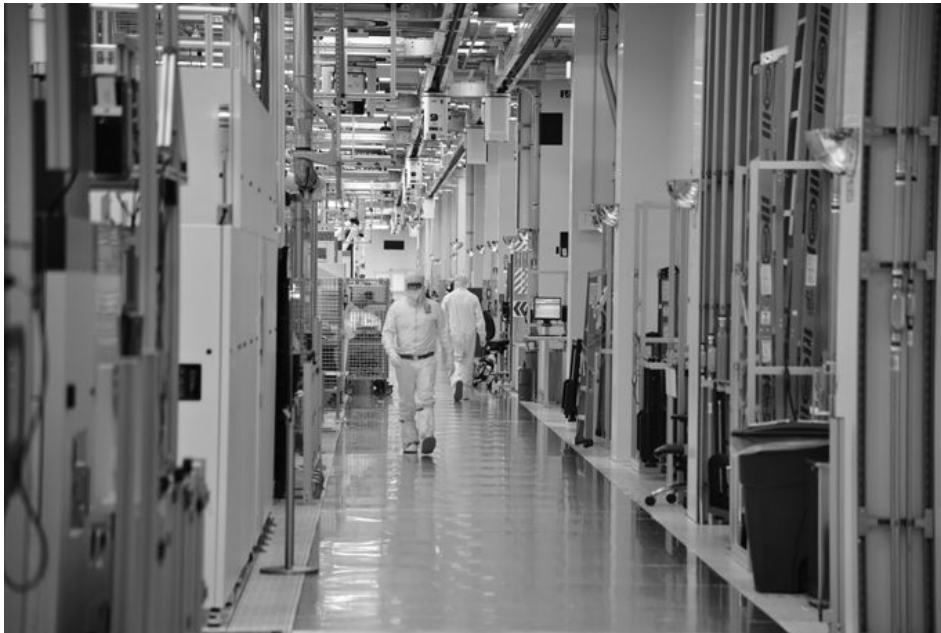
Figure 5.4 – Picture of a wafer fab; overhead delivery vehicles can be seen moving along their tracks (Courtesy of Intel Corp.)
