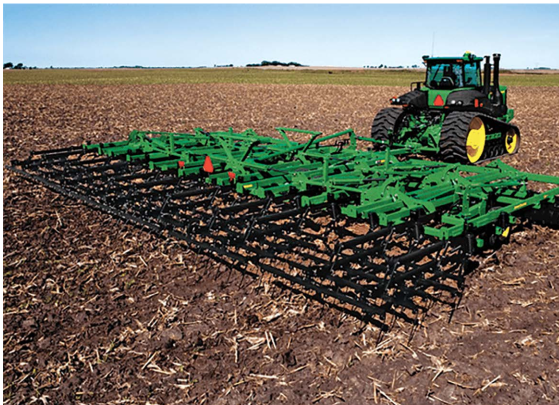
Fig. 13.2. Minimum tillage, 'mintil' in operation. The method saves much fuel over traditional deep ploughing.
