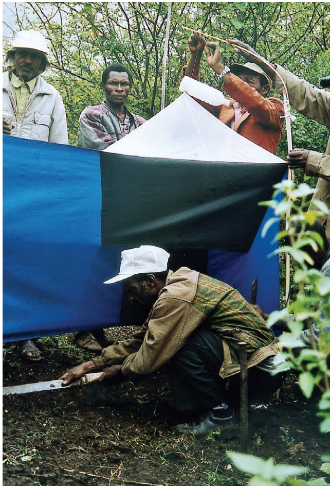
Fig. 13.4. The effective bi-conical trap for tsetse being set up in East Africa. Their slow reproductive rate makes them vulnerable to such methods of population reduction. Source: Flickr, credit to Peter Rickwood/IAEA.
