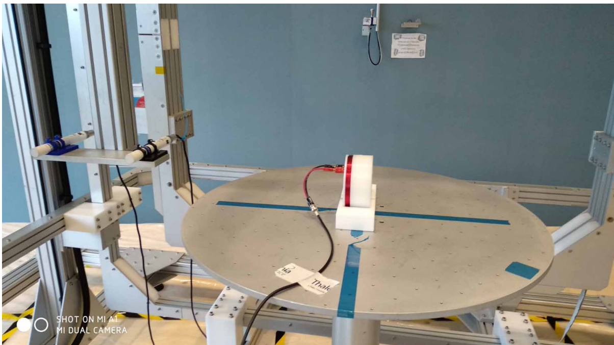
Figure 19. Magnetic Dipole Source in TAS-I Magnetic Coil Facility during validation measurements.
