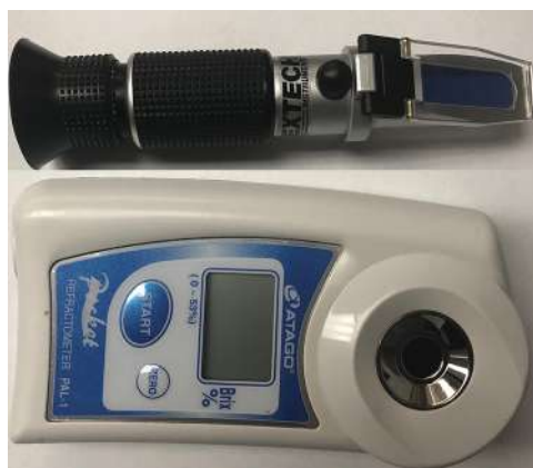
Fig. 14.8. Hand-held refractometers, digital (top) and manual (bottom). (Photos: Ali Sarkhosh.)
