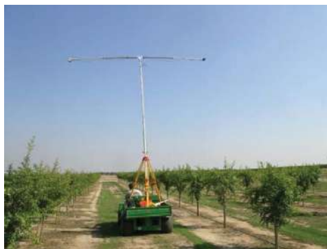
Fig. 10.2. Determination of canopy vigour in a young pomegranate orchard using a multispectral camera at the University of California Kearney Agricultural Center (KAC). (Photo: Claude J. Phene et al. , 2015, University of California Agriculture and Natural Resources.)
