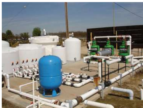
Fig. 10.7. Irrigation and fertilization equipment for applying fertigation in a pomegranate orchard. (Photo: Claude J. Phene et al. , 2015, University of California Agriculture and Natural Resources.)
