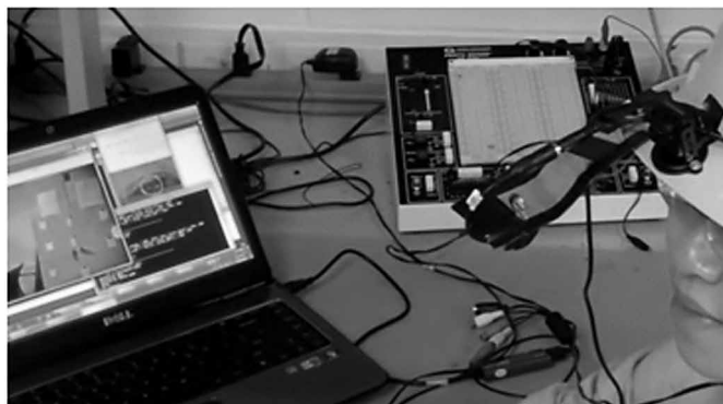
Figure 4. Head-mounted eye-tracker Source: The authors
