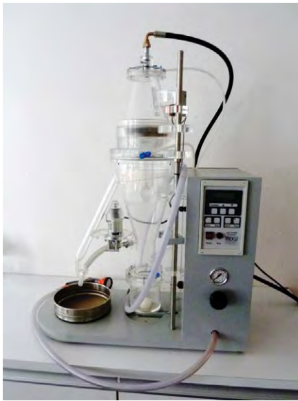
Fig. 2.9. Automated soil sample extractor for cysts. (Photo: JKI Münster, Germany.)
