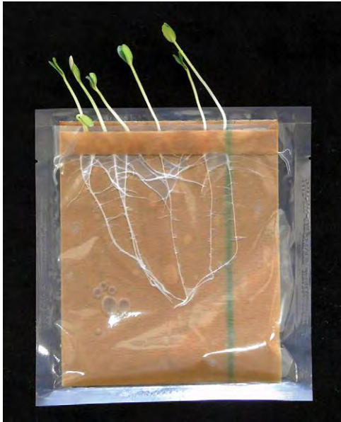
Fig. 10.5. Seed germination pouch with seedlings used to culture root-knot and cyst nematodes ( https://mega-international.com ) (Atamian et al. , 2012).
