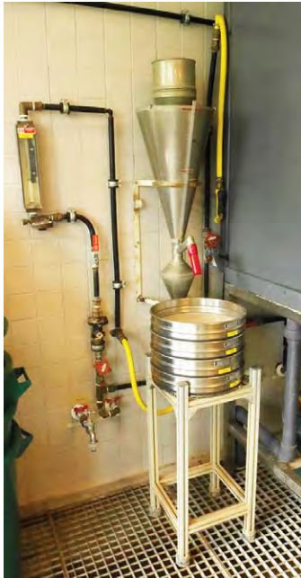
Fig. 2.18. Oostenbrink elutriator made of stainless steel with stack of four sieves. (Photo: ILVO, Merelbeke, Belgium.)
