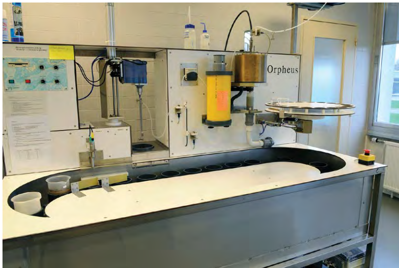
Fig. 2.2. Automated zonal centrifugation. The lower carousel feeds the samples to the centrifuge (1 l beaker) and the upper carousel receives the nematode suspensions (150 ml beaker) after the centrifuging process. The bowl of the zonal centrifuge is kept inside a metal cage for safety. The sample, kaolin (yellow vessel) and MgSO 4 (blue container upper right corner) are brought into to the centrifuge bowl through tubes. (Photograph, courtesy ILVO, Mellebeke, Belgium.)
