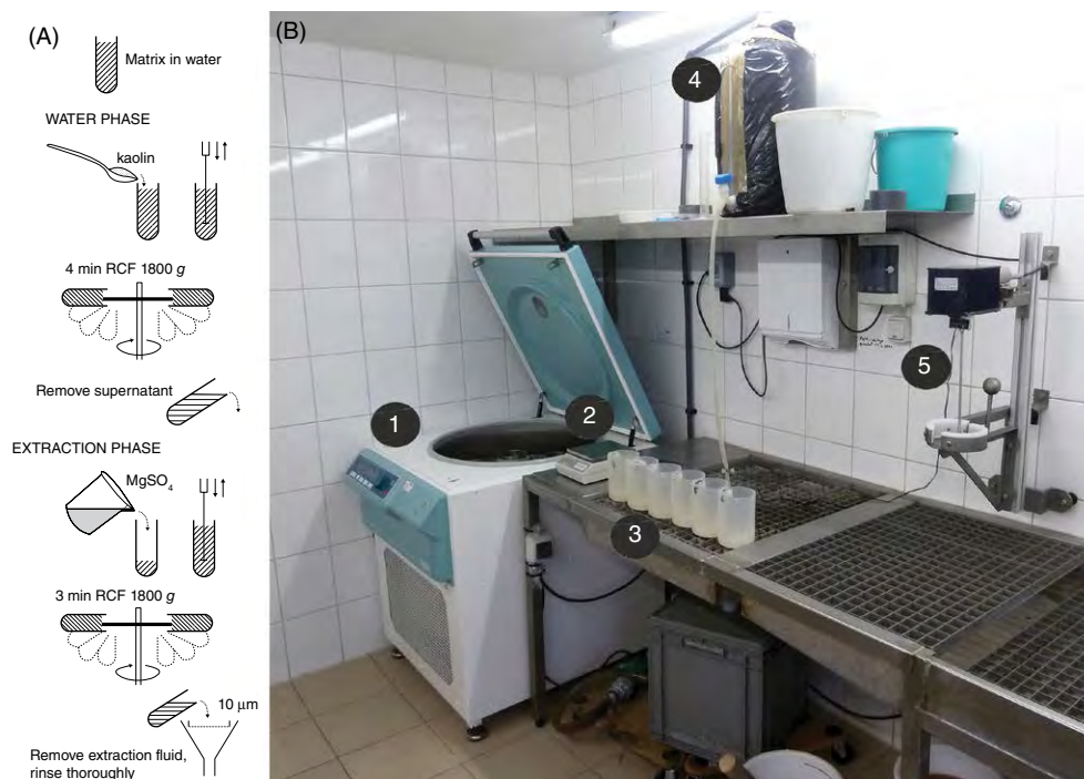
Fig. 2.1. (A) Schematic workflow of the centrifugal flotation method (after van Bezooijen, 2006). (B) Equipment used for centrifugal flotation: 1, centrifuge; 2, balance; 3, centrifuge tubes (1000 ml); 4, container with MgSO 4 solution; and 5, Vibro mixer. (Photo: JKI Münster, Germany.)
