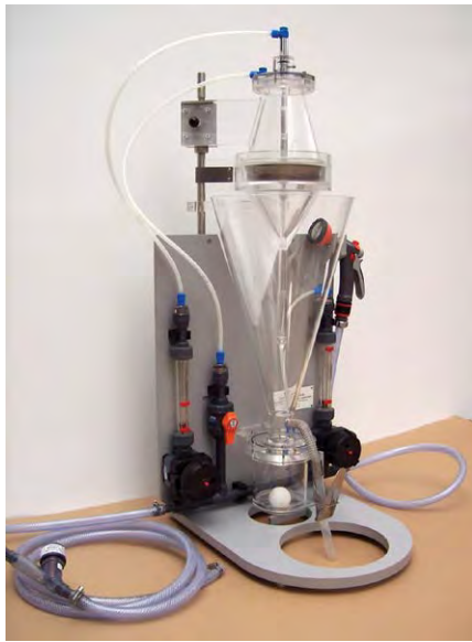
Fig. 2.19. Modified Oostenbrink elutriator made of acrylic glass. (Photo: MEKU GmbH, Germany.)
