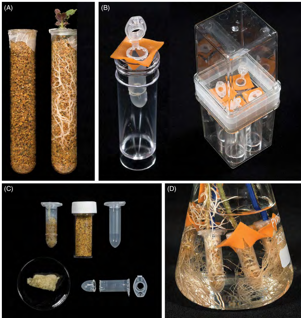
Fig. 6.5. Transparent containers for gnotobiotic cultures. (A) Boiling tube containing coarse substrate to grow potato chits. (B) Polystyrene universal container, Eppendorf snap-cap microcentrifuge tube, Magenta jars. (C) Eppendorf snap-cap microcentrifuge tube adapted to culture tomato on sand and rockwool. (D) Tomato roots. (Copyright Rothamsted Research Ltd.)
