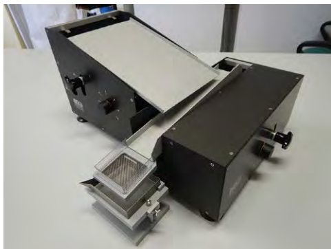
Fig. 3.5. Meku-Extractor for separation of cysts of Globodera spp. from organic float in dried samples. Two boards with roughened surface independently can be adjusted to an angle of 20° as well as intensity of vibration; round cysts roll down each board and dried float moves upwards where it can be collected in a chamber at the back of the device.
