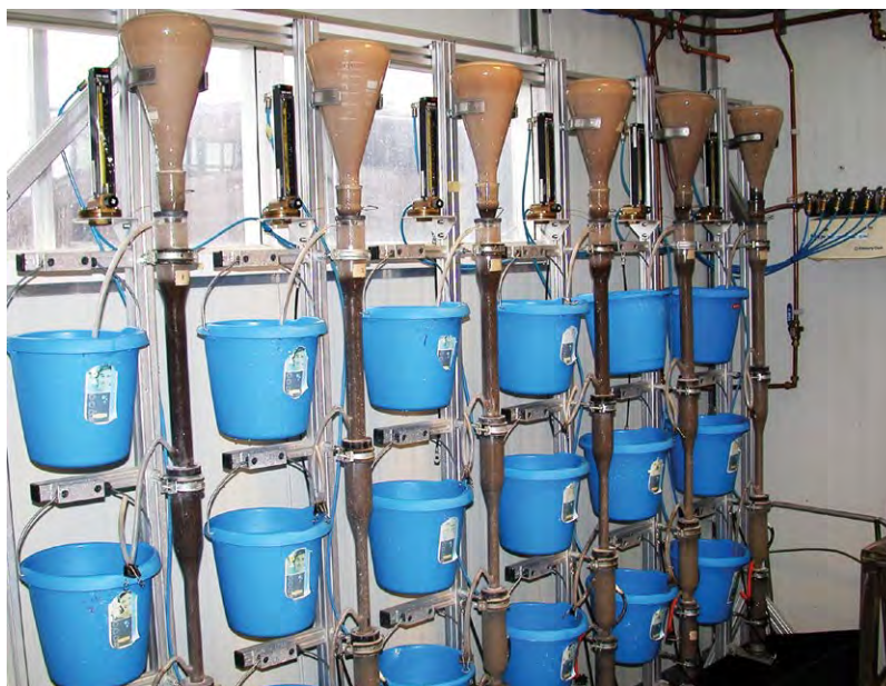
Fig. 2.22. A series of six identical improved Seinhorst elutriators, each with three buckets (I, II, III, top to bottom) and flasks installed on top. (Photo: Wageningen University and Research Centre, Wageningen, The Netherlands.)
