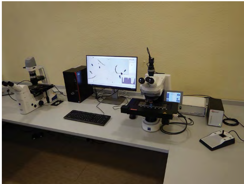
Fig. 3.4. Inverted (left) and compound (right) microscope equipped with scanning stage for eight slides, x-y-z-steering and high-resolution camera connected to a PC for automated image analysis of nematode suspensions.
