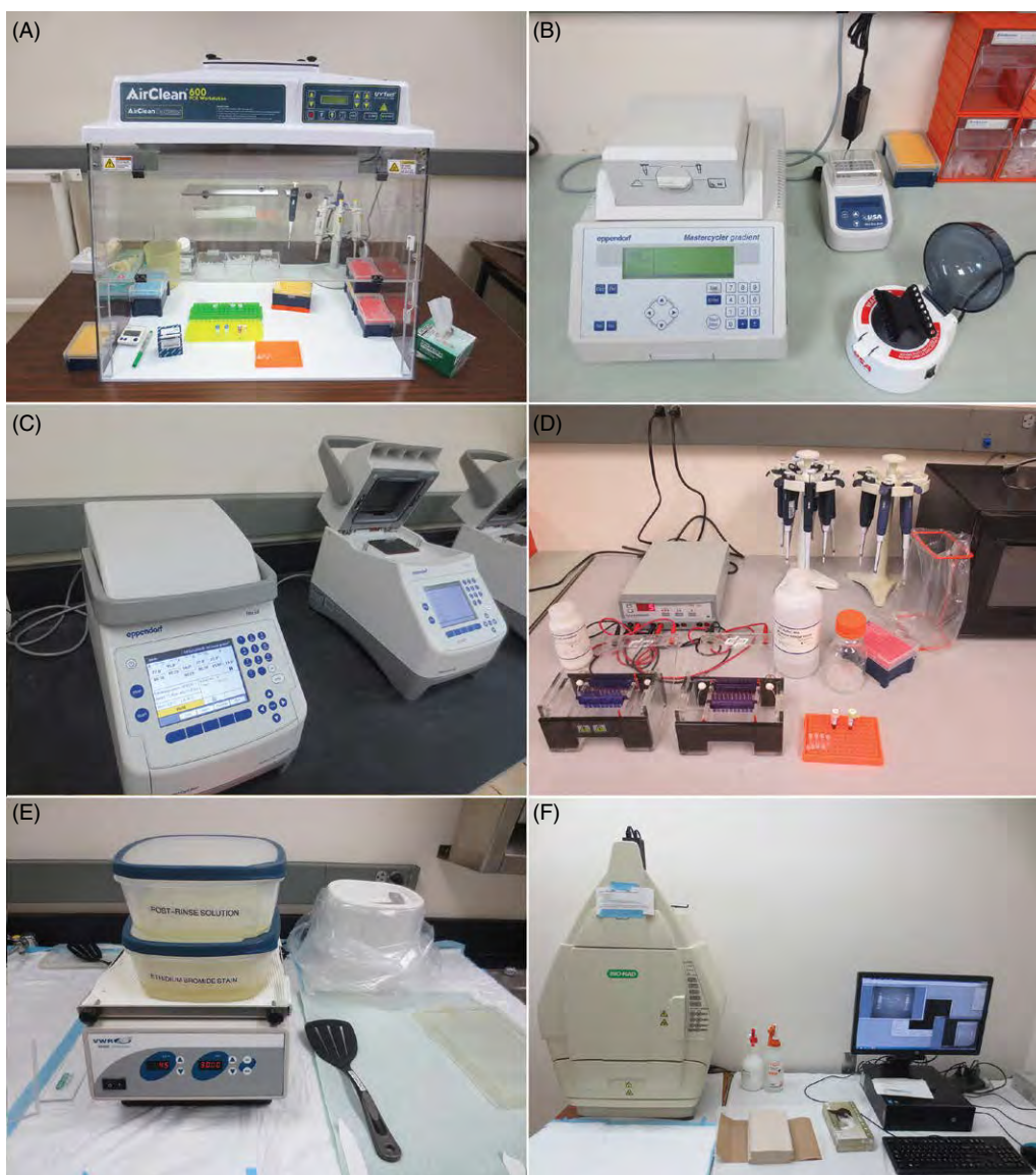
Fig. 12.1. Laboratory equipment. (A) AirClean PCR workstation for preparation of PCR mixture. (B, C) Eppendorf PCR thermocycles. (D) Gel electrophoresis supplies and equipment. (E) Containers for EtBr staining. (F) Bio-Rad gel imaging system.
