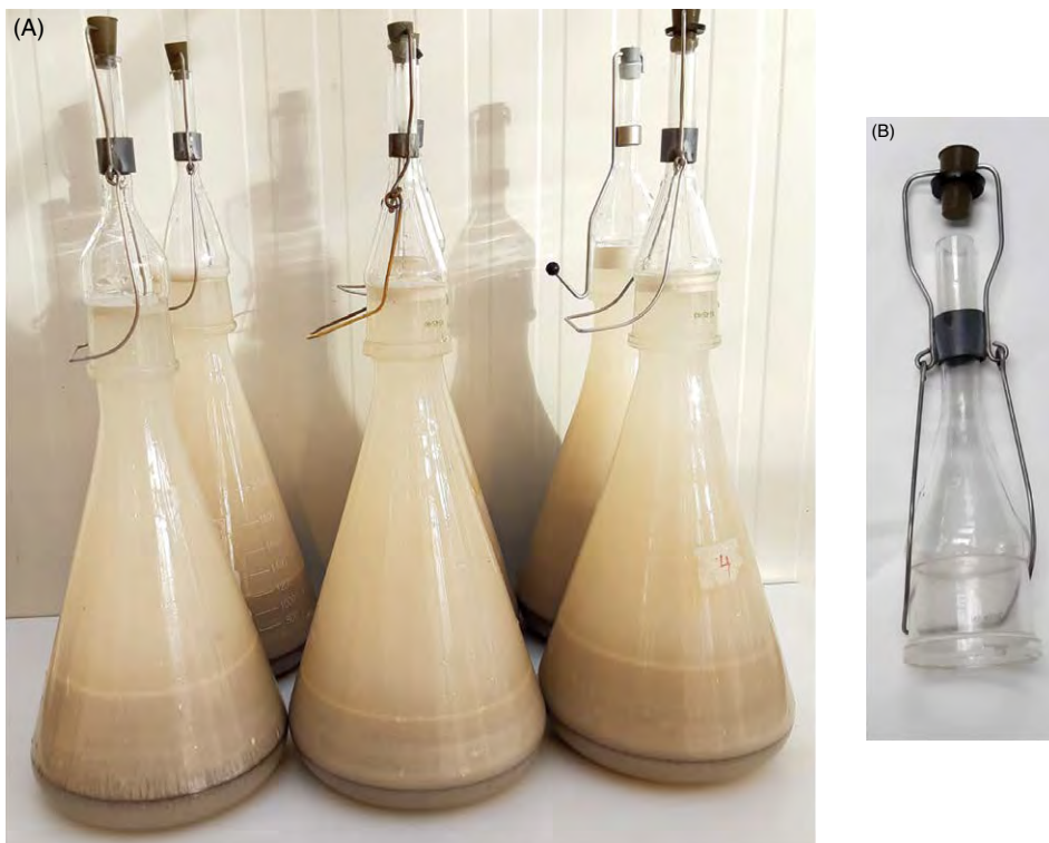
Fig. 2.20. (A) A set of six flasks with soil samples ready to be added on top of five improved Seinhorst elutriators. (see Figs 2.21–2.22). (Photo: Wageningen University and Research Centre, Wageningen, The Netherlands.) (B) The funnel-shaped mouthpiece with a stopper to close a flask before it is put upside down on the elutriator, where, once installed, it can be opened easily to release its content. (Photo: Wageningen University and Research Centre, Wageningen, The Netherlands.)
