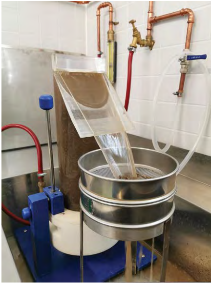
Fig. 2.11. Wye washer in action (Photo: FERA, Sand Hutton, UK.)
