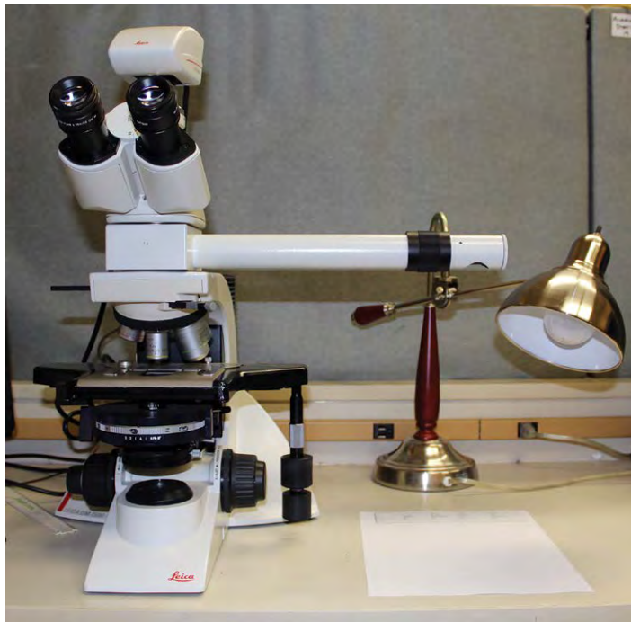
Fig. 7.3. Compound microscope equipped with a drawing tube and light source for measurement and drawing.
