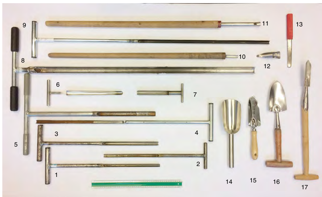
Fig. 1.3. Sampling tools; 1 to 9 are various sizes of augers. 1, 1.0 cm diam., 25 cm length; 2, 1.3 cm diam., 25 cm length; 3, 1.5 cm diam., 25 cm length; 4, 1.2 cm diam., 40 cm length; 5, 2.0 cm diam., 25 cm length; 6, 2.0 cm diam., 25 cm length; 7, 2.0 cm diam., 15 cm length; 8, 3.0 cm diam., 100 cm length; 9, 1.5 cm diam., 60 cm length; 10, 1.0 cm diam., 6 cm length; 11, 2.0 cm diam., 5 cm length. 8 and 9 are special augers for sampling potato cyst nematodes; 12 and 13 are tools for removing soil from augers; and 14 to 17 are small shovels and trowels in various sizes for taking soil and plant samples.
