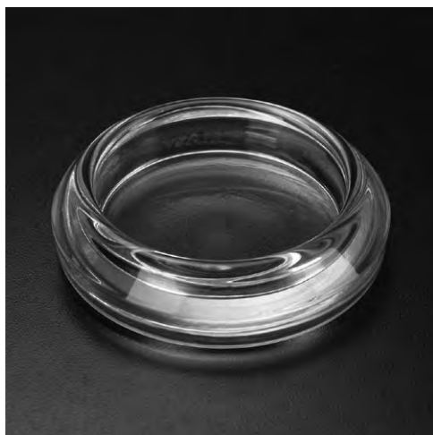
Fig. 5.4. A Syracuse watch glass; a Bureau of Plant Industry (BPI) dish is similar in shape but only 2.5 cm diam.
