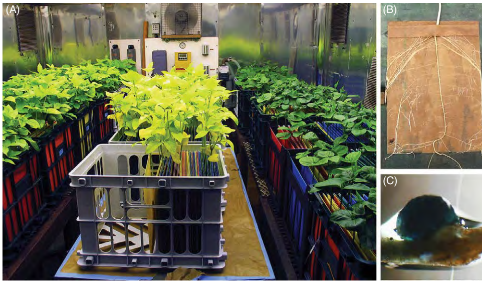
Fig. 4.2. The seedling growth pouch root-knot nematode screening system in a controlled environment chamber. (A) Young cowpea plants in seedling growth pouches arranged in hanging file folders following inoculation with Meloidogyne incognita second-stage juveniles. (B) Cowpea root system growing on the paper insert from a seedling growth pouch. (C) M. incognita egg mass on a root surface differentially stained blue with Brilliant Blue FCF (Erioglaucine) 35 days post inoculation. (Photographs courtesy of Philip A. Roberts, University of California Riverside, USA.)
