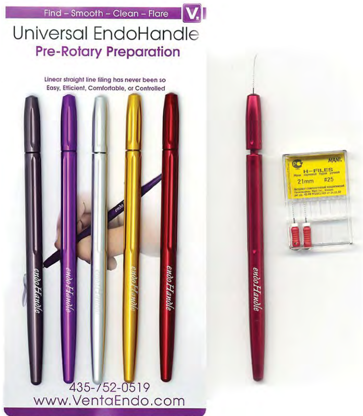
Fig. 5.1. Package of five universal endohandles that are useful holders for the endodontic H-type files (left) and a single handle with an attached H-type #25 file (21 mm long) that has been sanded smooth with a sharpening stone and slightly curved to make a nematode handling pick.
