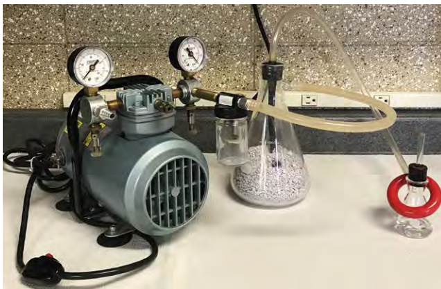
Fig. 11.4. Vacuum pump used to remove gas molecules from the acrylamide solution.
