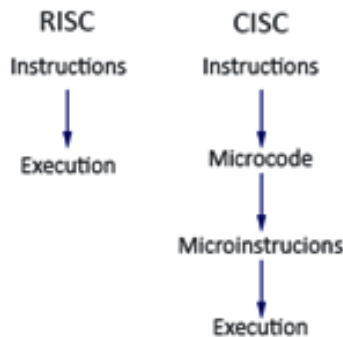
Figure 1.8 – Difference between RISC and CISC
