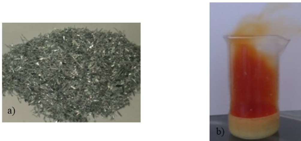
Figure 3.7 Zinc dissolution: a) Zinc chips; b) Zinc dissolution reaction.
