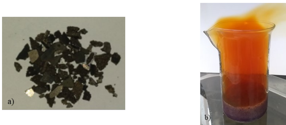
Figure 3.8 Manganese dissolution: a) Manganese chips; b) Manganese dissolution reaction.
