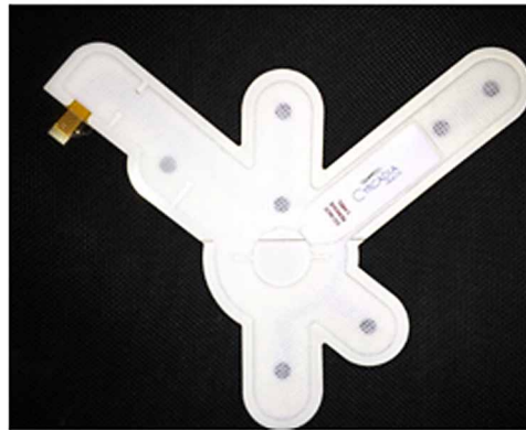
Figure 9. Seven sensors positioned within the bra ( https://www.arrow.com )
