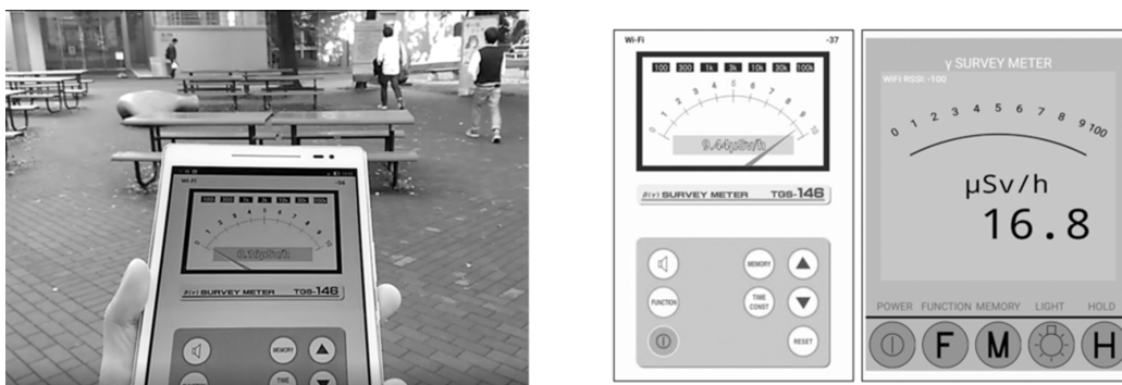
Figure 5. USOTOPE in use: terminal with the application running (left), screen captures of two types of measuring instruments emulated by the application (right)
