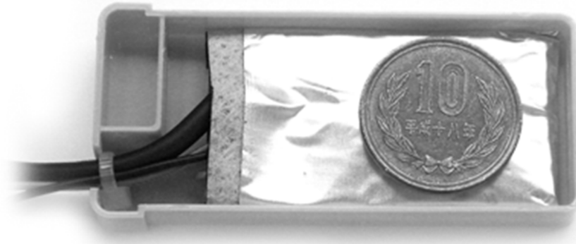
Figure 2. Assembling the Pokéga Type 1. The user places the Pokéga board in the mint candy case and uses a 10-yen coin as a shield against beta radiation.
