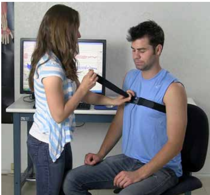
Figure 9.1 The Placement of a Respiration Belt Transducer. Source: Image courtesy of Biopac.
