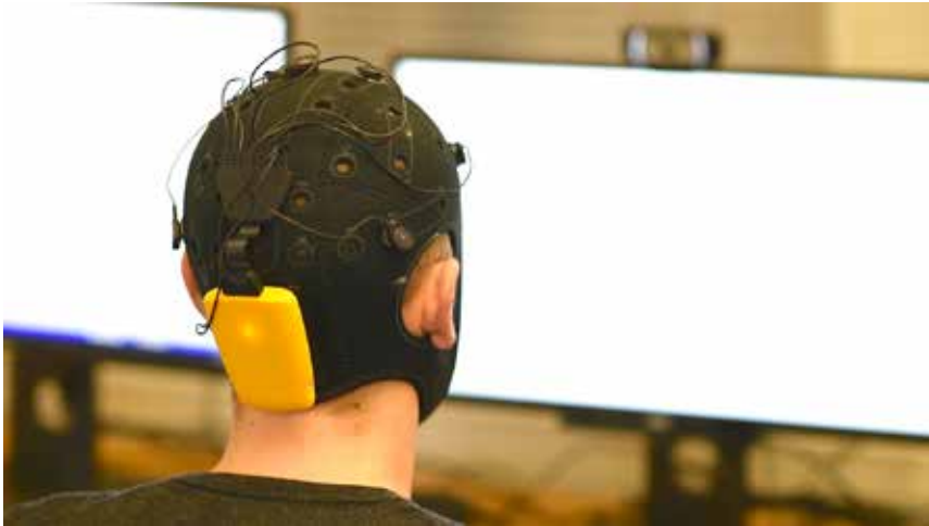
Figure 6.1 EEG Headcap for Wireless EEG Measurement. This Study Participant Is Wearing an EEG Headcap for Wireless EEG Measurement and Recording for Mobile Applications (by Enobio EEG Systems). Source: Image courtesy of iMotions, Inc.
