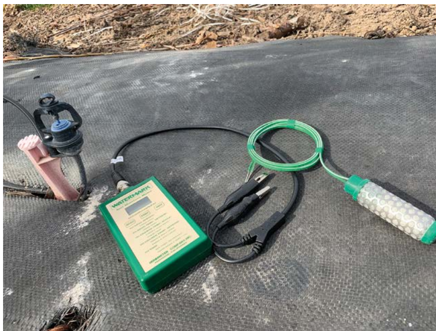
Fig. 8.1. Granular matrix sensors (GMS) are easy to install and give a fairly accurate reading of the soil moisture levels in the immediate vicinity of the probe (courtesy of L.E. Long).
