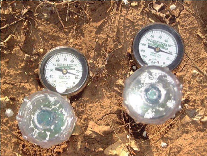
Fig. 8.3. These tensiometers are reading soil moisture at two different depths (courtesy of C. Kaiser).
