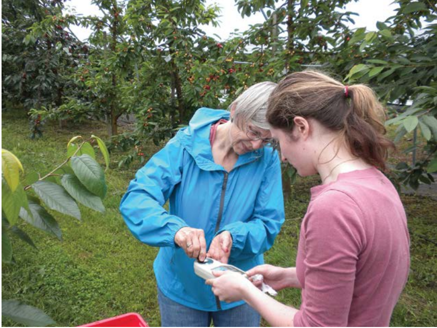
Fig. 9.10. A hand-held refractometer can help the grower make important harvest decisions (courtesy of L.E. Long).
