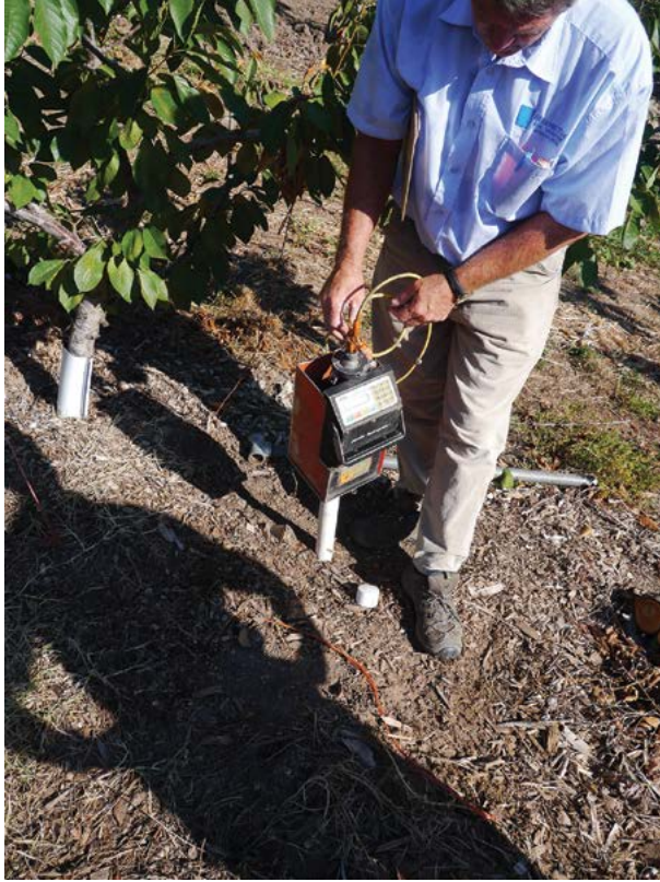
Fig. 8.2. Neutron probes are extremely accurate, but require a special license to operate (courtesy of L.E. Long).
