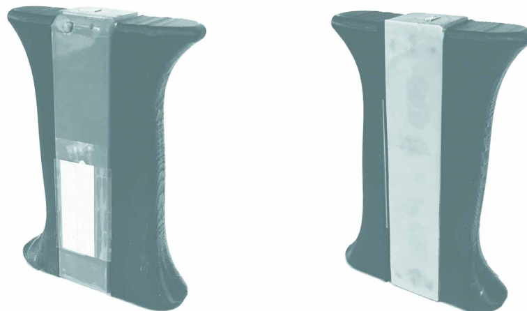
Figure 1. BodyGrip, muscle strength and energy measuring device
