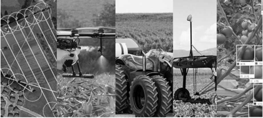
Figure 7.6: Outdoor agriculture robots: (a) spraying and weeding robots, (b) auto steering, (c) autonomous navigation, and (d) fruit harvesting robotics.
