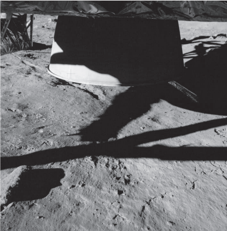
Figure 5-2. Smoothed soil beneath the Apollo 11 LM after landing. The engine bell is visible at the top of the image. Features indicative of soil erosion are visible in the image, including erosional remnants and a terrace where a natural lamination in the soil resisted erosion. The gouge in the soil at the top of the image is from the LM's soil contact probe (from NASA image no. AS11-40-5921HR).
