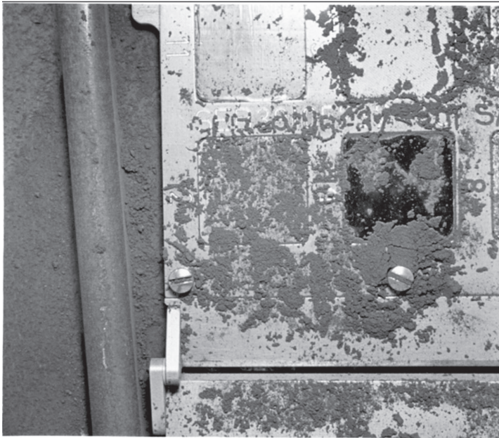
Figure 4-2. TDS showing the strong cohesion of lunar dust dislodged from the serial number on the mounting plate (Photo credit: NASA).
