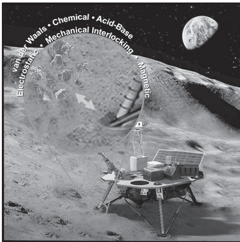
Figure 13-1. Lunar dust will interact with exposed surfaces through a myriad of mechanisms. Image credit: Susanne Waltz, Media Fusion.
