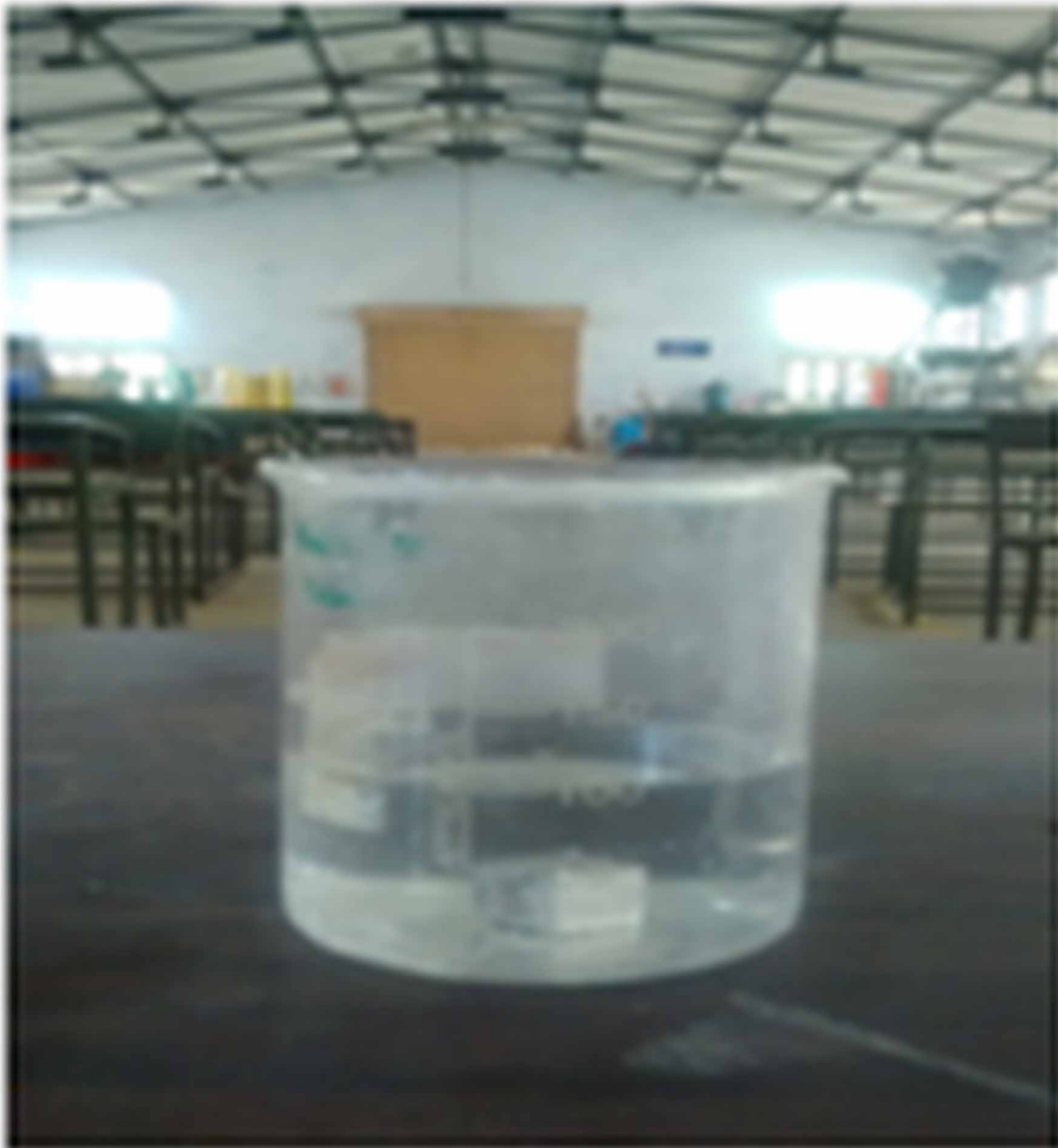
Figure 8. Immersion corrosion test
