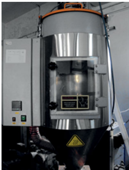
Fig. 2: Dehumidifier for preheating of the fillers.
