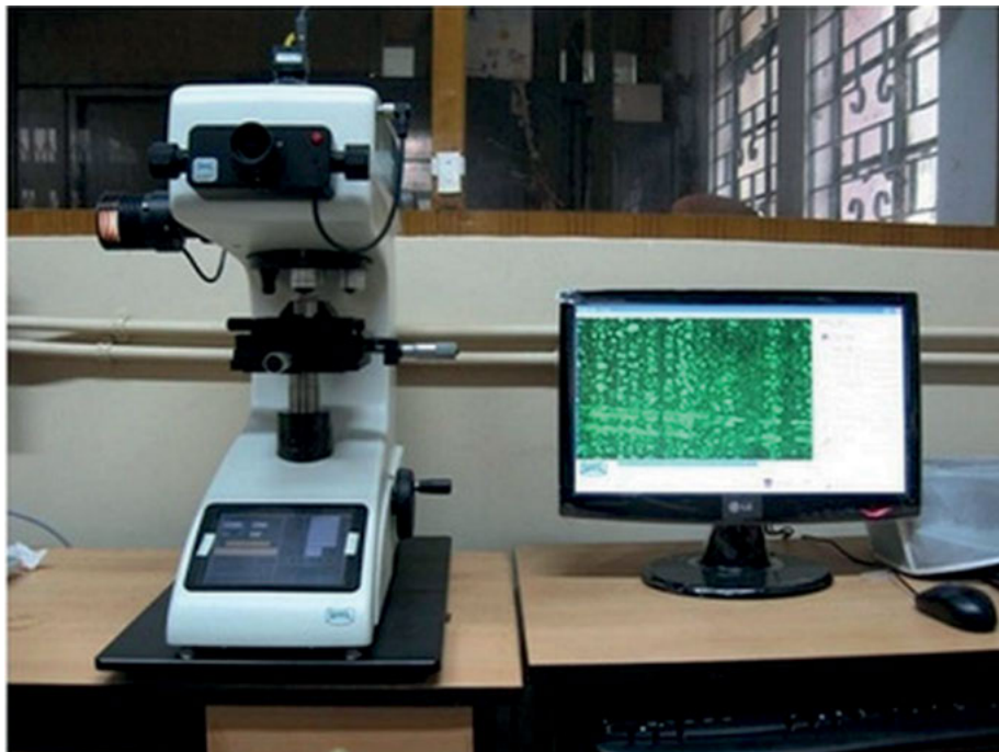
Fig. 7: Vicker's hardness test setup.
