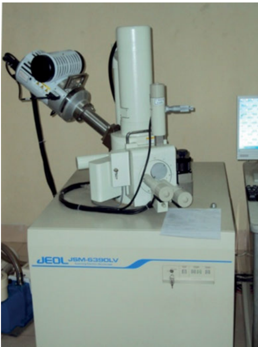
Fig. 8: Scanning electron microscopy setup.
