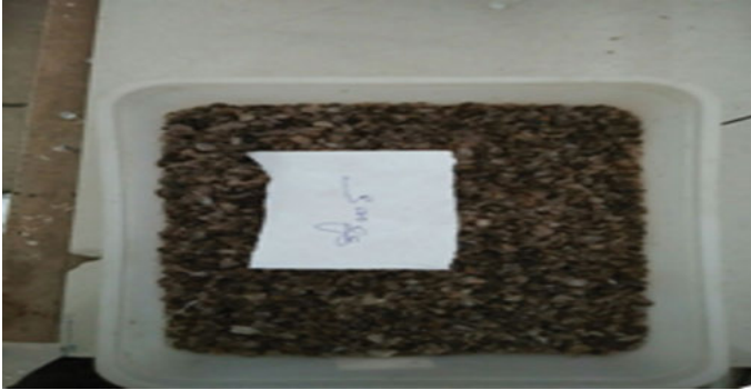
Fig. 15: Ground granules of coir and PPE.
