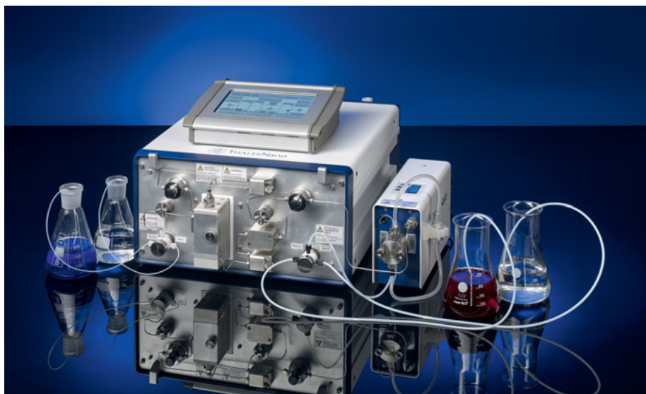
Figure 6.12: ThalesNano's H-Cube Pro. The system consists of a high-pressure pump, a hydrogen generator, a heated reactor with the catalyst inside, and a back-pressure regulator. The system can be operated at temperatures up to 150 °C and can supply hydrogen at pressures up to 100 bar.
