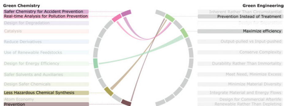
Figure 9.3: The application of process analytical technology (PAT) addresses multiple principles of green chemistry (prevention, less hazardous chemical synthesis, real-time analysis for pollution prevention, inherently safer chemistry for accident prevention) and green engineering (maximize efficiency, prevention instead of treatment).
