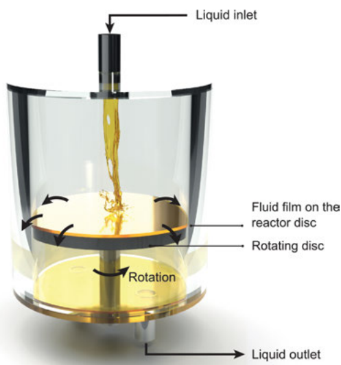
Figure 5.10: Schematic of a spinning disk reactor is designed for very fast liquid/liquid reactions with large heat effects such as nitration, sulfonation, and polymerization.
