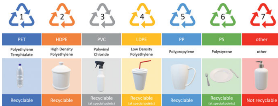
Figure 1.4: Resin identification codes (RICs) according to the coding system of the Society of the Plastics Industry (SPI).
