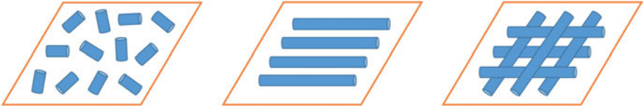
Figure 2.62: Various types of fiber orientation (blue) in composite matrix (orange): (a) random, (b) unidirectional, and (c) bidirectional.
