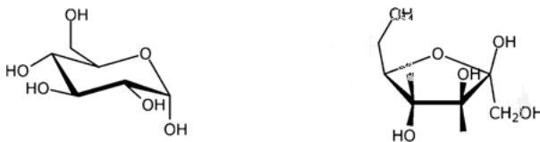
Figure 3.18: Chemical structures of glucose (left) and fructose (right).
