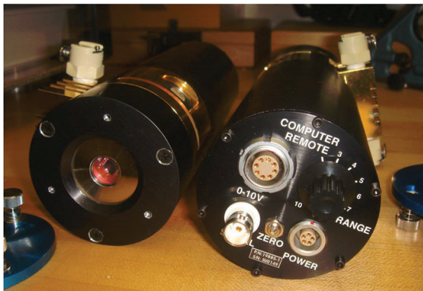
Fig. 28. Picture of water-circulated and 4-stage TE cooled 5-mm extended-InGaAs detector/radiometer standard.
