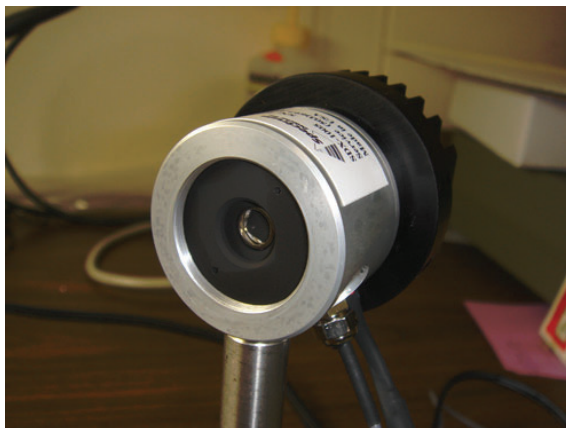
Fig. 36. Picture of a temperature-controlled low-NEP pyroelectric hybrid detector standard.
