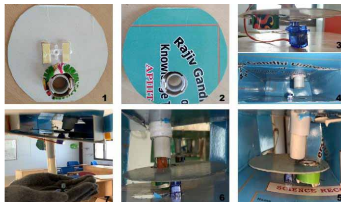
Figure 4. Circular disk with servo motor holder, circular disk, circular disk with servo motor, cylindrical tube for loading, overall box with mechanism, loading objects, releasing objects
