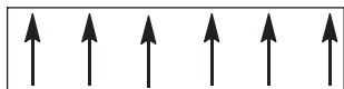
Figure 6.7: Alignment of neighbouring spins due to unpaired electrons in the same direction in ferromagnetic materials.
