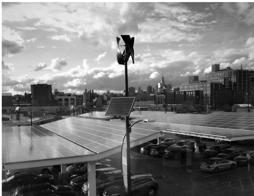
Figure 6.1. Solar panels and wind turbine over a supermarket car park in New York. Photo by the author.
